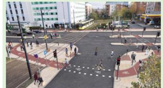
Junction improvements for cyclists and pedestrians (CYCLOPS junction, Greater Manchester)
